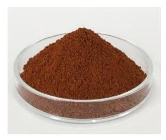
A high efficiency iron composite catalyst able to generate hydrogen through the DMR reaction. The catalyst is superior both in initial activity and sustained activity.
