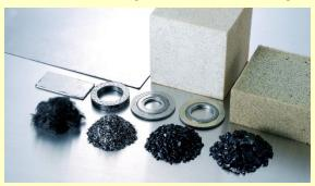
Thermally expandable graphite (TEG) developed by ATN Graphite Technology K.K. has superior flame and chemical resistance and is widely used for car parts and construction materials. Trial operations of the new plant began in April 2022. It aims to improve production efficiency and develop applications in the electronic materials field and other fields
