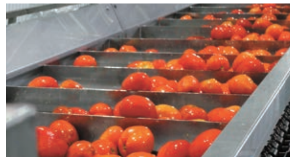
Tomato washing process in the juice production line at Gold-Pak Co., Ltd.'s Eniwa Plant
