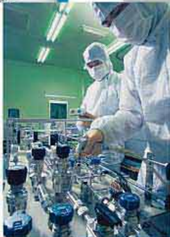
Fabrication of gas supply systems for semiconductor production
