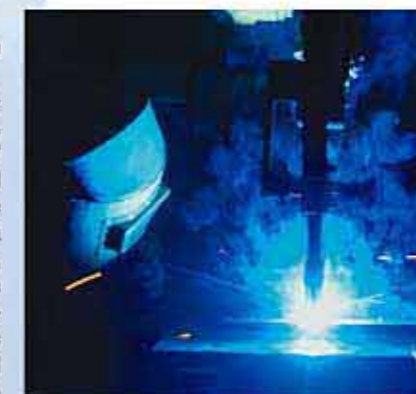
"ELNACKS" welding by a welding robot
