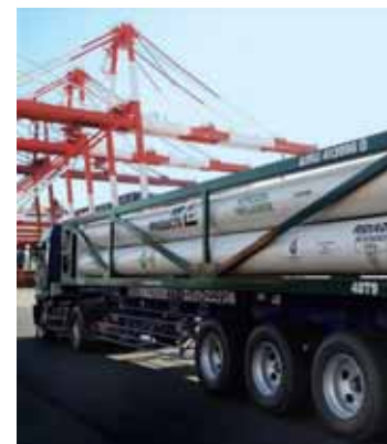
Nitrogen Trifluoride ISO Module (40 foot)
