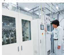
PFC Collection, Refining and Recycling system
