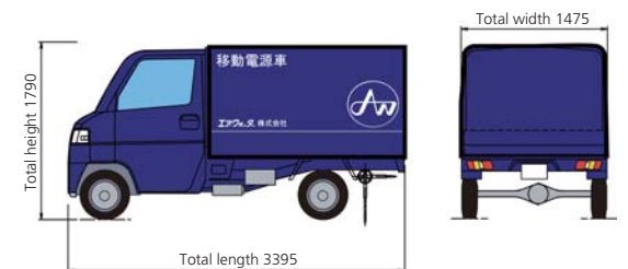
Compact mobile power source car
