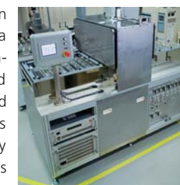
Atmospheric Pressure Plasma continuous hydrophobic treatment system
