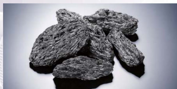
Needle coke that is the raw material in electric furnace electrodes
