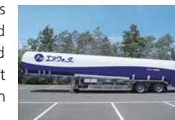
15.7-ton LNG tank truck with one of the largest LNG shipping capacities in Japan
