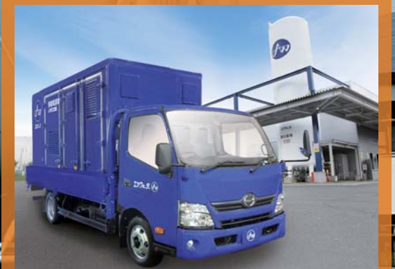
50 kW LP gas-type mobile power source car
