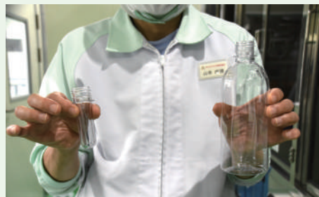
Plastic bottles on the aseptic filling line are formed from test tube-size preforms and use half the amount of plastic compared to regular plastic bottles
