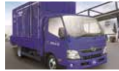
LP gas mobile power supply vehicle
