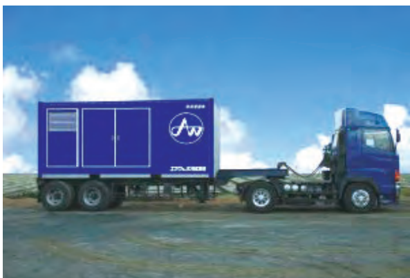
Vehicle-mounted electricity generator powered by LP gas
