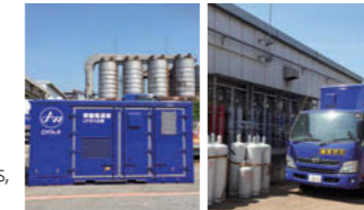
Power source cars dispatched during a blackout
